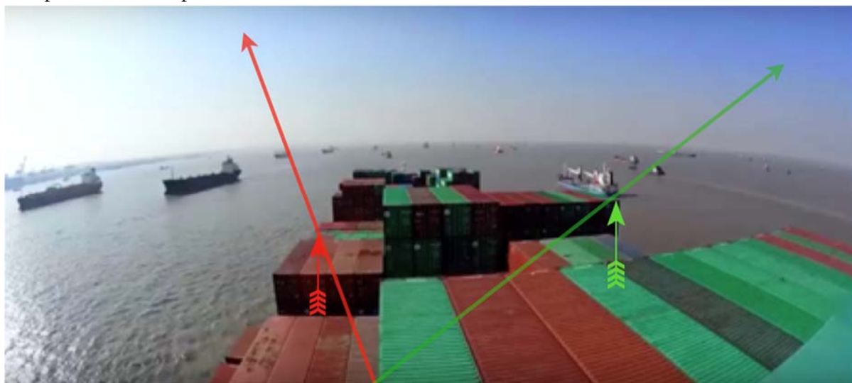
Figure 1-06-1: use deck cargo as reference mark for movement check
